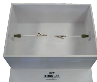
ALLIGATOR CLIPS FOR SECURING INTERNAL STRUCTURE
